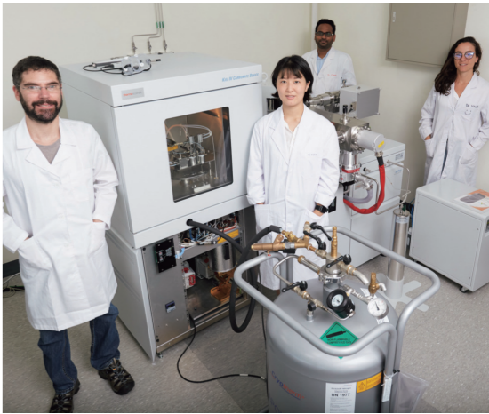
Figure 4. The Mat 253 Plus IRMS coupled to the Kiel IV automated carbonate preparation device with Porapak filter system.
